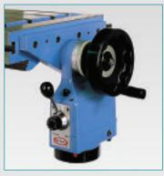
**SERVO X SERVO Y** Electronic "SERVO" feed unit
