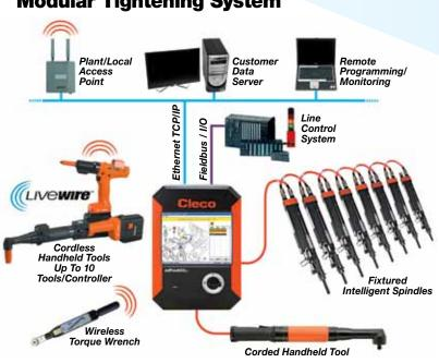
One controller manages up to 32 tools simultaneously in varying combinations.
