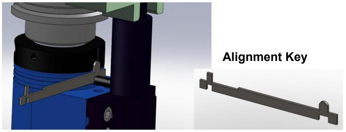
Adjustment of the Alignment Collar: With the TapWriter in the machine spindle and the stop arm engaged with the stop location next to your machine spindle, orient the machine spindle to the tool change position. Bring the slot in the alignment collar in line with the tab of the stop arm. There is a small alignment key included with the tool to help you to line this up. Tighten the collar's clamping bolt very securely.
