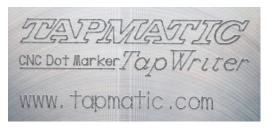
Marking plane 3mm, 850 RPM, 500 mm/min.
