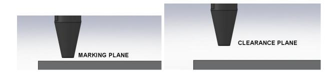
A safe starting point for marking steel (for example AISI 4130 at 30 HRC hardness) with 1/4" (6 mm) high characters is as follows: 750 RPM spindle speed, 50 in/min (1270mm/min) feed rate (X +Y axis), Rapid speed or 400 in/min (10,000mm/min) lift-off and down-feed (Z-axis), 0.250" (6mm) Clearance Plane, 0.070" (2mm) Marking Plane. Below are some recommended programming parameters.
