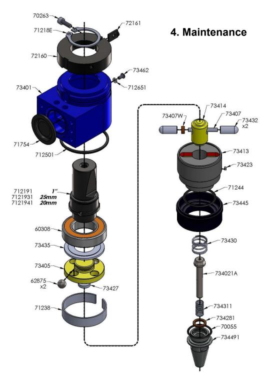
**Changing Stylus and Springs:** You can easily replace the stylus, stylus spring or hammer spring by simply unthreading the Nose Cone 27 from the bottom of the housing. Be sure not to lose O-Ring 26, during this procedure.
