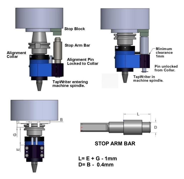
You may also use the alternative installation shown above using a stop block. Please let us know whether the distance from the centerline of your machine is 55mm, 65mm, or 80mm and we can supply the correct assembly for your machine.
