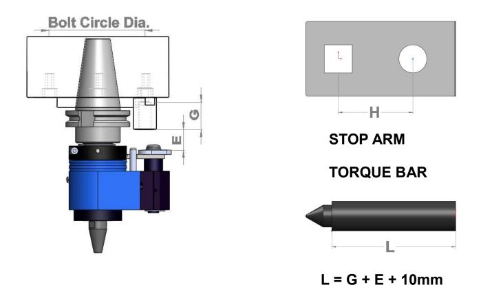
**Modifying or selecting the Stop Arm**: The TapWriter comes with a blank stop arm that can be modified to fit the bolt circle of your machine.
