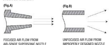
Air exiting from an improperly designed nozzle diffuses outward 3 to 4 times wider than the air-jet from the patented AIR-SPADE supersonic nozzle. (Fig.B)
