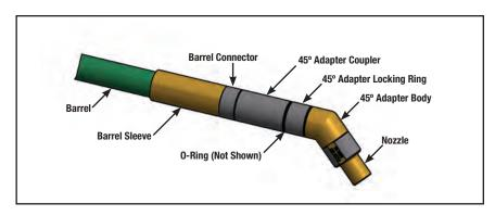
CAUTION: When using the 45° adapter, compressed air exiting the nozzle will force the tip of the tool away from the direction the nozzle is aimed. To prevent this from occurring, the operator should place the free hand at least midway down the barrel. Grip the barrel tightly to brace the tool against the force produced by the exiting compressed air.
