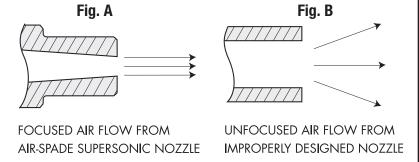
Air exiting from an improperly designed nozzle diffuses outward 3 to 4 times wider than the air-jet from the patented UTILITY AIR-SPADE supersonic nozzle. (Fig.B)
