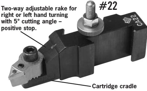
Tool Steel Cartridge adjusts every 15° for right or left hand turning, facing or chamfering. 12 positive lock positions. Exclusive positive lock with 2-way force holding insert down and tight against shoulder. Standard triangular carbide insert has 6 cutting edges.
