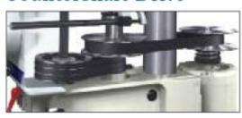
Three V-belts and a cog belt transmit positive power to the spindle.
