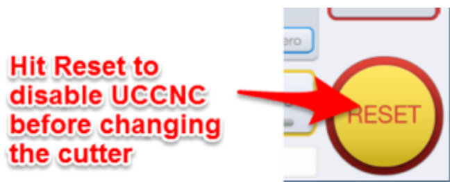
Figure 12: Reset to disable spindle relay
