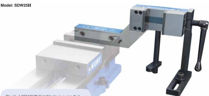
The Kurt SDW25II SideWinder is a vise that mounts vertically to the back of any Kurt industry standard 6" vise. The SideWinder includes a stabilization leg that will mount to the table on the movable end of the vise and a workstop to position the height of the part.
