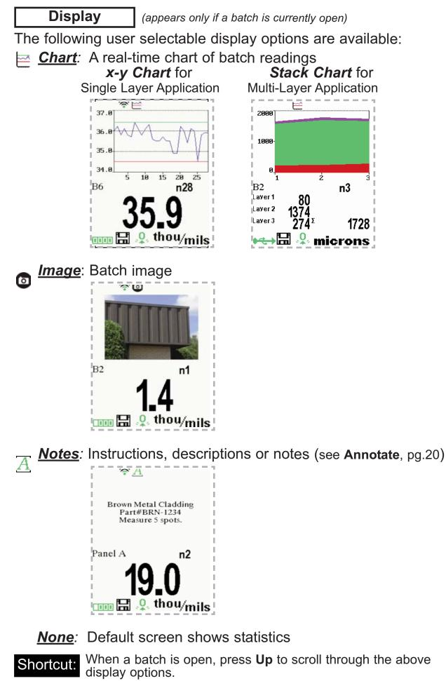
**NOTE:** PosiSoft.net (pg. 24) and PosiSoft Mobile (pg. 25) are used to insert an *Image* and *Notes* into a batch.
