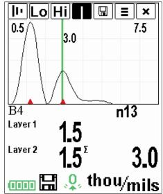
These interfaces are depicted by a "peak". The greater the change in density, the higher the peak. The more gradual the change in density, the greater the width of the peak. For example, two coating layers made of essentially the same material and "blended" would result in a low, wide peak. Two materials of very different density and a well-defined interface would result in a high, narrow peak.
