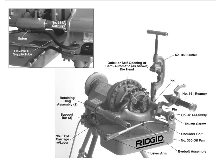
NOTE! Disconnect Power Drive from power source before mounting No. 311A Carriage onto Power Drive.
